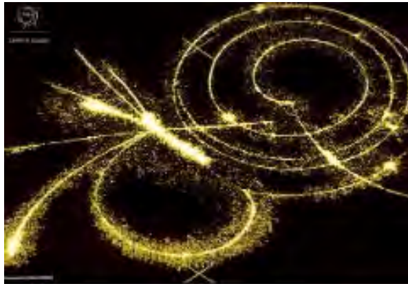
Antiproton interactions with neon nucleus in the streamer chamber
